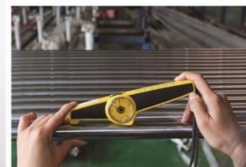
Inspection of piston rod coating
