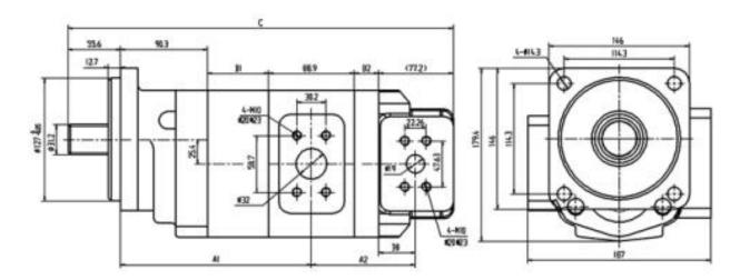
A1=134.7+(B1/2) A2=82.4+B2 B1=12.7+tooth width B2=12.7+tooth width C=312+B1+B2
