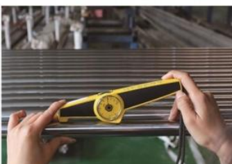
Inspection of piston rod coating
